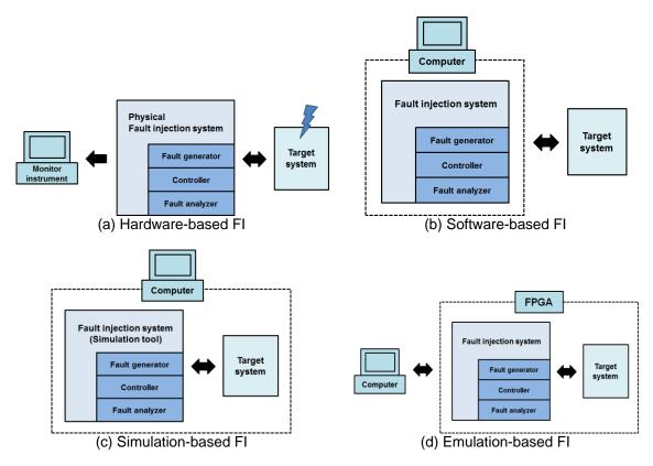
Figure 3. Fault Injection Techniques
