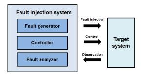
Figure 2. Fundamental environment of the FI method
